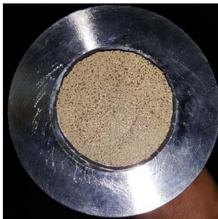
Potted 4-in fiber module cross-section (early design)
